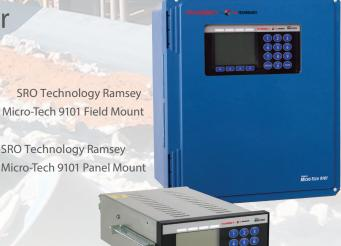
The Micro-Tech 9101 scale integrator electronics provides the intelligence to the weighing system, integrating output signals from the weighbridge and speed sensors to arrive at a rate of material flow and total material passed over the scale. The electronics also functions as the system power supply and incorporates all features that allow calibration, operation and diagnostics for the system.
