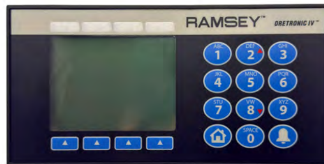
Figure 1-8. TMD IV Control Unit Keypad
